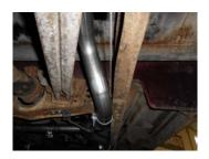
4) Take the **86076** muffler inlet pipes and place a supplied 2½" clamp onto the expanded end, place them onto the back of the H-pipe assembly's **86074** & **86075**. Rotate them up into their approximate position and tighten the clamps enough to hold but still allow for adjustment.
