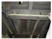
7) To mount the rear tailpipe hangers on short bed trucks, measure forward 17½" from the rear of the frame, there will be a factory hole mid-way up the frame rail. Using the 3/8" hardware provided, and bolting through the bottom hole of the **HA572** hanger installed on the tailpipe hanger, bolt the hanger to the side of the frame. Be sure the **HA572** is straight up and down then drill a 3/8" hole through the top hole in this hanger and secure with a 3/8" bolt, nut and washers.
