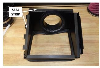
11. Cut the adhesive seal strip (6) to the lengths required, and apply it to the four edges of the heat shield.
