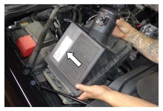
If your VECI label is affixed to the stock airbox (as shown in the example above), a replacement label must be obtained and affixed to a suitable location in the engine compartment. Replacement VECI labels can be ordered from the dealership or from on-line suppliers. Be prepared to provide your VIN number, since the label is VIN number-specific.
