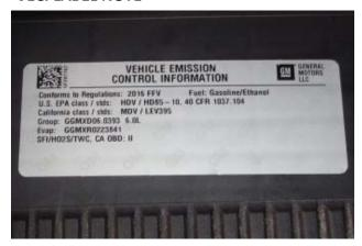
California emissions law requires the Vehicle Emission Control Information (or VECI) label to be readily-visible in the engine compartment.
