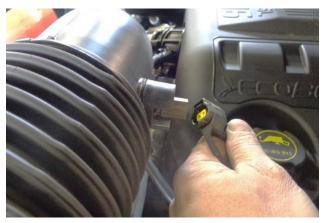
5. On the back of the intake duct, disconnect the inlet air temperature sensor plug.
