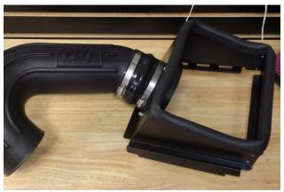
13. Assemble the intake tube (13) and heat shield.
