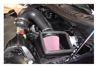
16. Insert the four tabs on the heat shield into the slots on the back of the airbox. Lower the intake tube and slip the two couplers over their turbo ducts. Do not tighten the clamps at this time.
