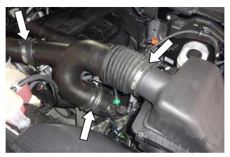
4. Loosen the screw clamps on the 3 ends of the air intake duct.
