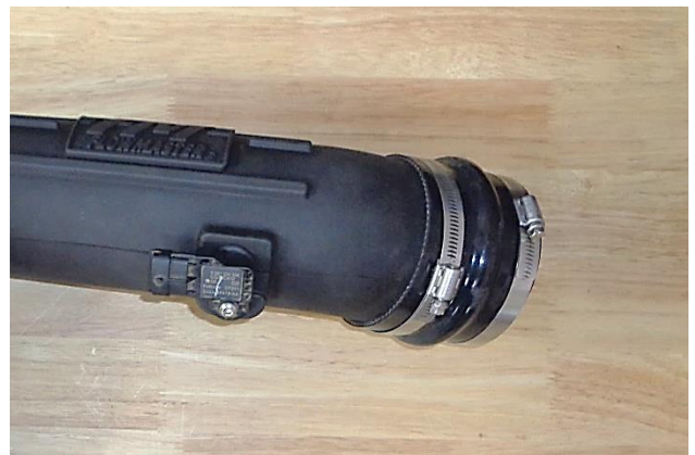
17. Slip the two remaining screw clamps (10) onto the other 4" flex coupler (11). Push the coupler onto the intake tube, and snug – do not tighten – only the tube clamps at this time. (Leave the other clamps loose.)
