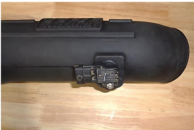
14. Install the grommet (12) in the intake tube (14). Then install the sensor in the grommet using the M6 screw (9). (Soapy water will ease insertion of the grommet in the tube, and the sensor in the grommet.)
