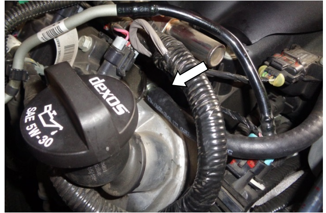
22. Push one end of the 5/16" ID hose (27) onto the metal tube from which the PCV line was disconnected at Step 7.
