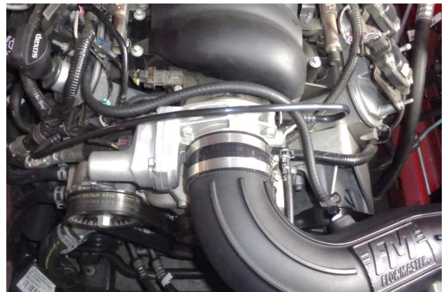
23. Route the hose across the top of the throttle body, below the hard plastic line, and to the barbed fitting. Cut the hose to length, and use the pinch clamp (28) to secure it to the fitting.
