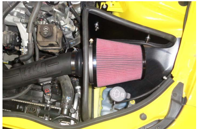
23. Install clamp (2) on air filter (1), install filter on filter adapter and tighten clamp.
