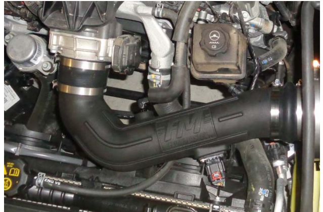
22. Install assembled intake tube in vehicle and tighten all hose clamps.
