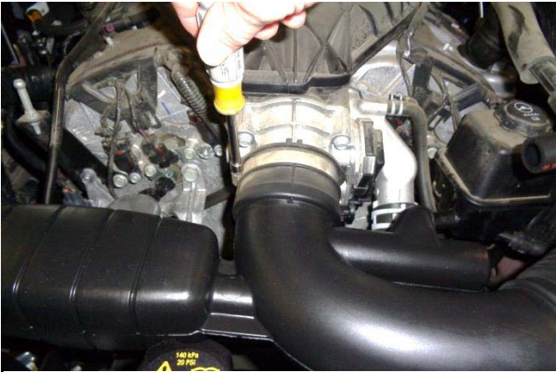
8. Loosen the hose clamp that secures the intake tube to the throttle body.
