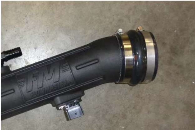
19. Install 2 hose clamps (20) on flex (or humped) coupler (19), then install coupler on intake end of intake tube. Orient clamp screws upward to allow tightening after installation on vehicle.
