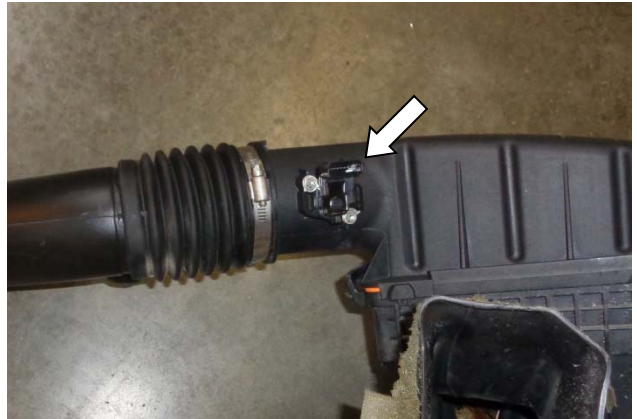
11. Remove the MAF sensor from the intake tube, then remove the factory gasket from the sensor. CAUTION: The sensor is delicate! Handle with care, and store in a safe location until reinstallation.
