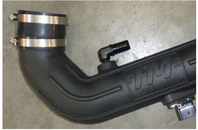
21. Install 2 hose clamps (26) on straight coupler (27), then install coupler on discharge end of intake tube. Orient clamp screws upward to allow tightening after installation on vehicle.
