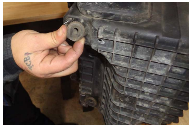
12. Remove any two of the four rubber grommets from the bottom of the airbox, for use at Step 18 .
