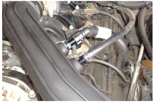
27. Connect the PCV and / or EVAP hoses to their respective fittings, as applicable. Verify that the PCV connector is securely latched to the QD fitting. Secure the EVAP hose to the barbed fitting with the pinch clamp (14).
