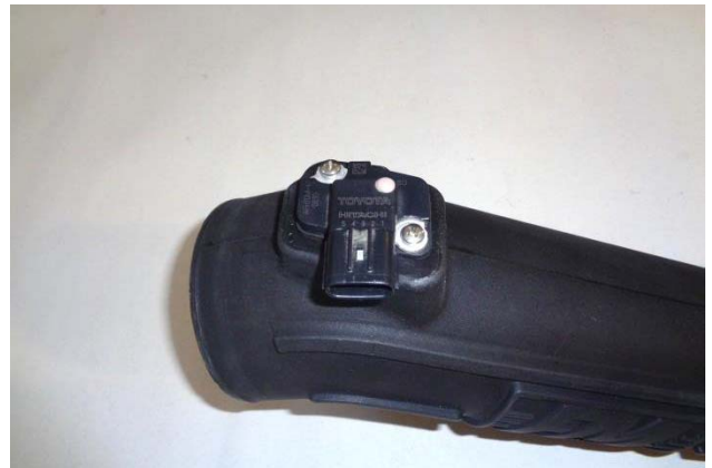
24. Install MAF sensor gasket (12) onto the sensor, ensuring correct orientation. Then install sensor in intake tube, using M4 screws (13).
