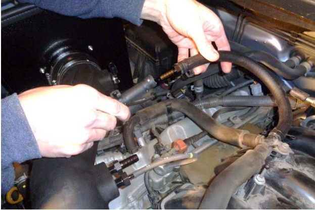
31. Install PCV hose (16) on barbed fitting and secure with pinch clamp (14).
