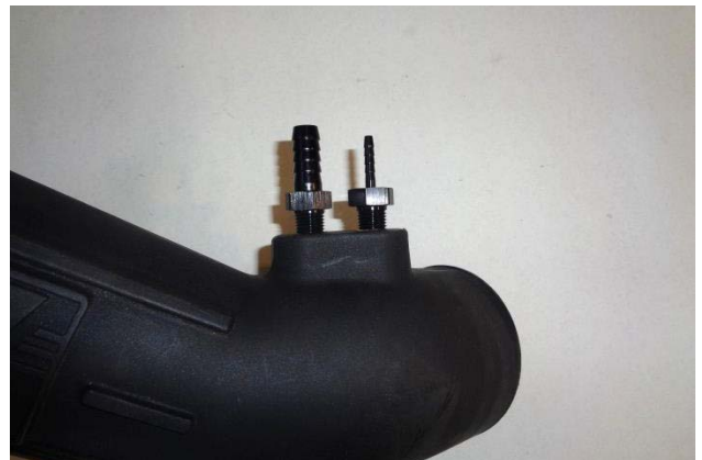
23. Apply 2 wraps of nylon thread tape to threads of barbed fittings (17) and (18), and install them in intake tube (19).
