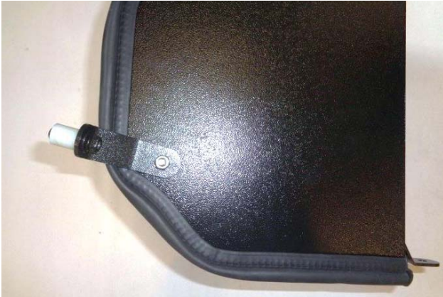
19. Attach bracket (26) to airbox using \frac{1}{4} -20 \times 5/8" screw (28) and flat washer (25) (against airbox), and nut (7) and lock washer (8) (against bracket). Leave bracket slightly loose until installation of airbox.
