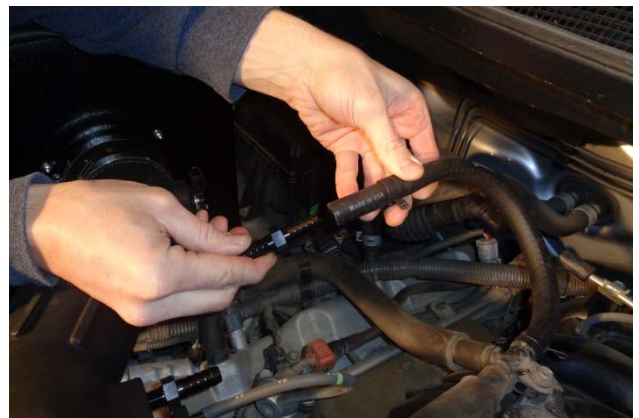
30. Insert barbed fitting (15) into PCV hose and secure with pinch clamp (14).
