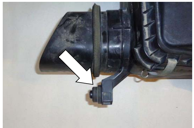
12. Remove the rubber bushing and retain for reinstallation.
