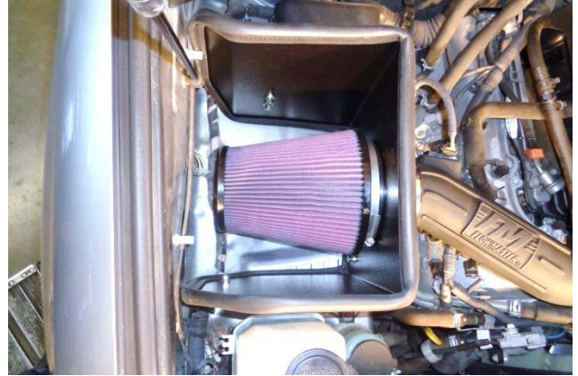
34. Install clamp (2) on air filter (1), install filter on filter adapter and tighten clamp.
