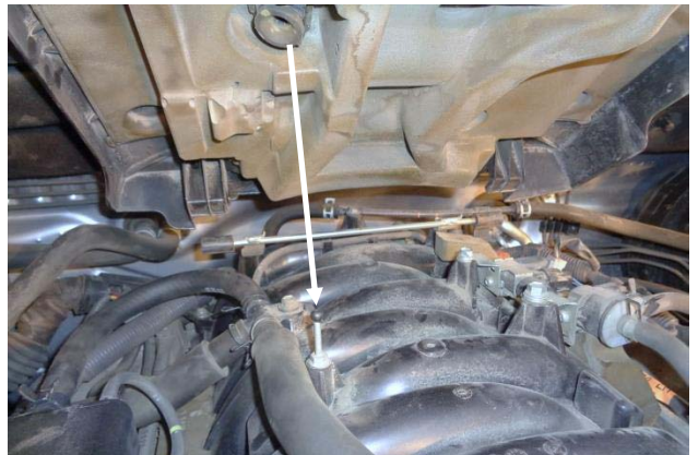
35. Install engine heat shield. Place clips at rear of cover on hinge bar, then lower the cover and snap it into place on the mounting post.
