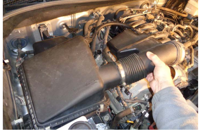
10. Remove the intake duct from the throttle body, then remove the assembled airbox and duct from the vehicle.
