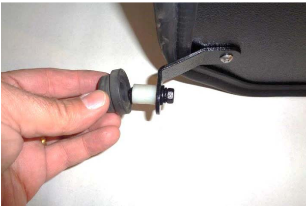
20. Attach nylon spacer (27) to bracket using \frac{1}{4} -20 \times 1/4" screw (24), lock washer (8) and flat washer (25) (against bracket), and nut (7) (against spacer). Install rubber bushing on spacer.
