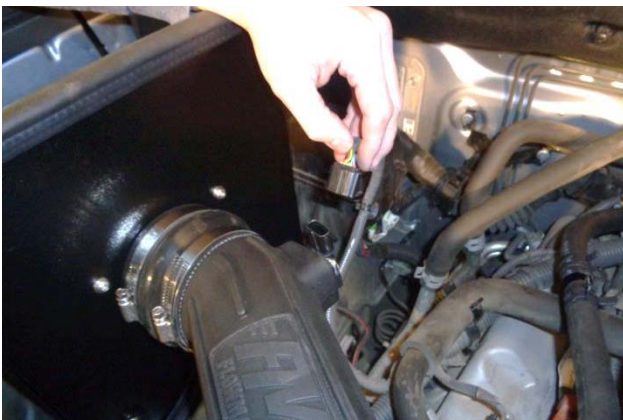
33. Reinstall the connector on the MAF sensor and verify that it is secure.
