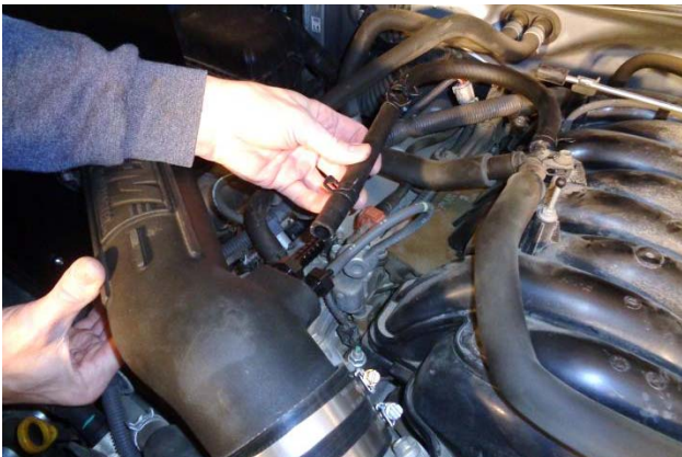
32. Install other end of PCV hose on barbed fitting in intake tube and secure with pinch clamp (14).
