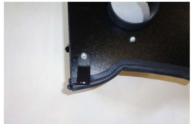
18. Attach bracket (24) to airbox using \frac{1}{4} -20 \times 5/8" screw (3) and flat washer (4) (against airbox), and nut (7) and lock washer (6) (against bracket). Leave bracket slightly loose until installation of airbox.
