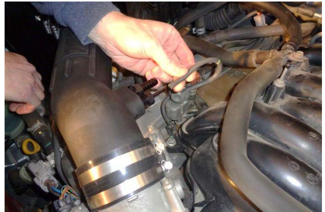
29. Install vacuum hose on small barbed fitting.
