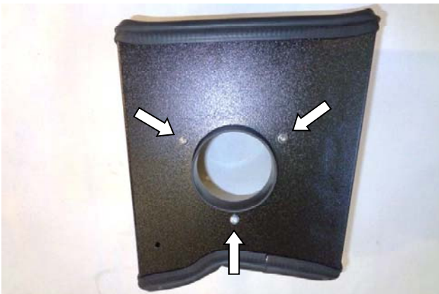
15. Assemble air filter adapter (29) to airbox using M6 screws (9), lock washers (10) and flat washers (8).
