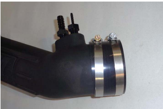
27. Install two hose clamps (20) on straight coupler (19), and install coupler on discharge end of tube. Orient clamp screws so as to allow tightening after installation on vehicle.
