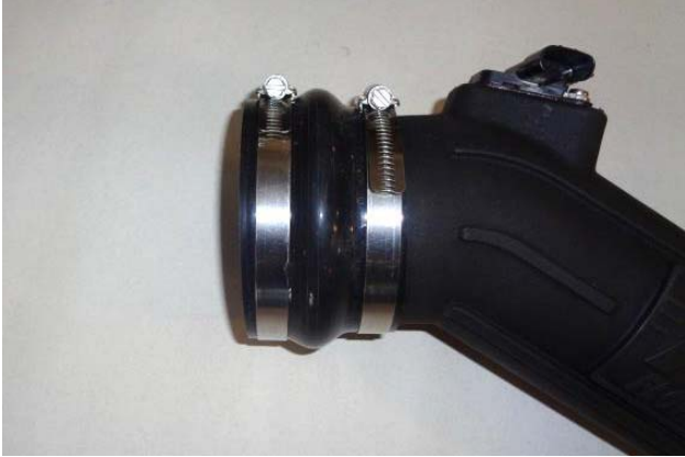
25. Install two hose clamps (22) on flex coupler (23), and install coupler on intake end of intake tube. Orient clamp screws to allow tightening after installation on vehicle.
