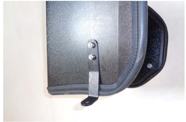
16. Attach bracket (5) to airbox using \frac{1}{4} -20 \times 5/8" screws (3) and flat washers (4) (against airbox), and nuts (7) and lock washers (6) (against bracket).
