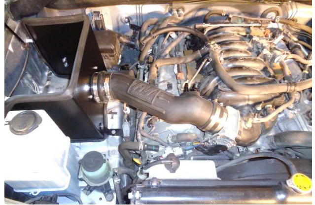
28. Install assembled intake tube in vehicle and tighten all hose clamps.
