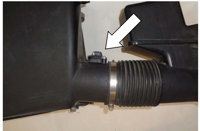
11. Remove the MAF sensor from the airbox, then remove the stock gasket from the sensor. CAUTION: The sensor is delicate! Handle it with care, and store it in a safe location until reinstallation.
