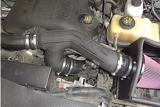
18. Install the intake tube in the vehicle, slipping the couplers over the two turbo inlets and filter adapter.
