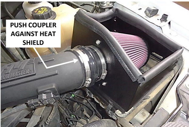
19. Push the right coupler up against the heat shield, then tighten only the filter adapter clamp at this time.
