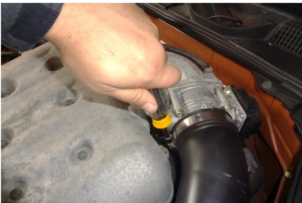
9. Loosen the screw clamp that secures the duct to the throttle body.
