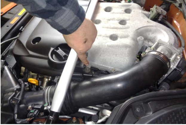
7. Remove the air duct bracket bolt.
