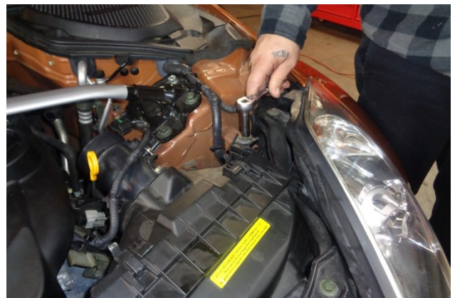
12. Remove the bolt that secures the airbox to the vehicle and retain it for use at Step 21 .
