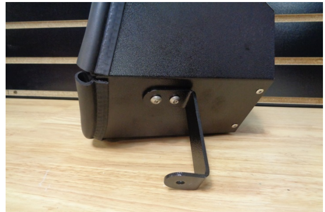
17. Attach bracket (16) to the heat shield using ¼-20 screws (7) (on the bracket side), and flat washers (4), lock washers (5) and nuts (6) (on the heat shield side).
