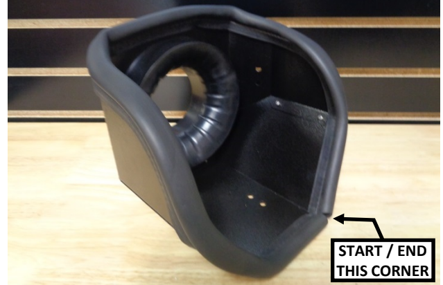
16. Attach the gasket (23) to the heat shield. Starting at the corner shown, firmly press the gasket onto the edge, gradually working around the heat shield. When you return to the starting corner, trim the gasket to fit using metal-cutting shears.
