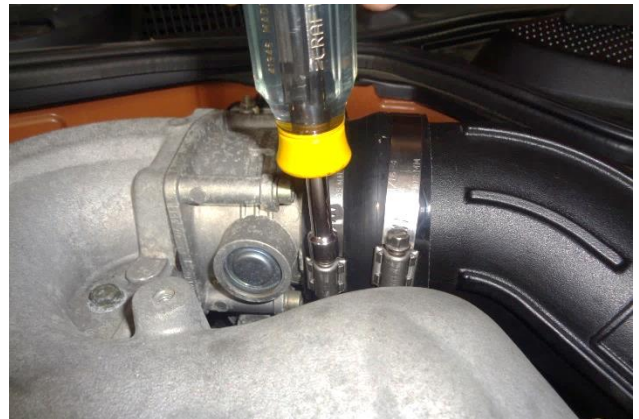
29. Tighten only the throttle body clamp.
