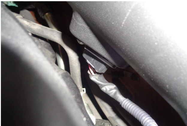
26. Push the MAF sensor plug onto the sensor until the locking tab clicks, then check the plug for security.
