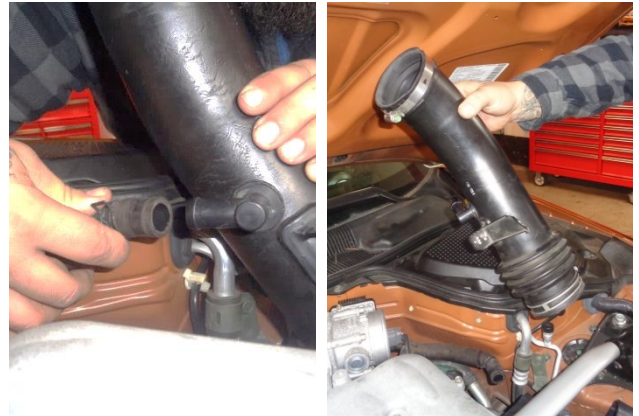
11. Loosen the pinch clamp, separate the PCV line from the intake duct and remove the duct from the vehicle. Retain the pinch clamp for use at Step 27 .
