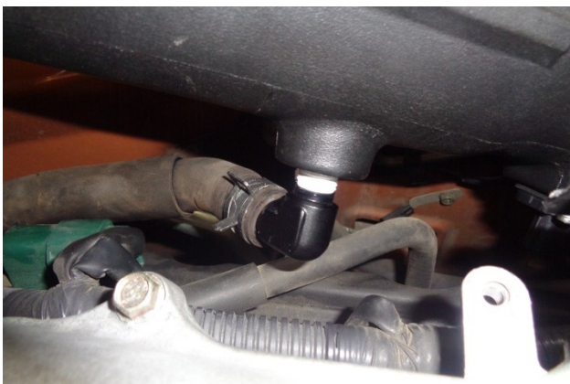
27. Push the PCV hose onto the elbow, and secure it using the stock pinch clamp (removed at Step 11 ).
