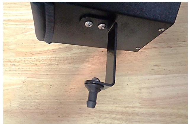
18. Attach the barbed pin (15) to the bracket using an M6 screw (11), lock washer (10) and flat washer (9).
