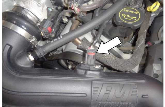
28. Reconnect the MAF sensor plug to the sensor, close the locking tab, and verify the connection is secure.
