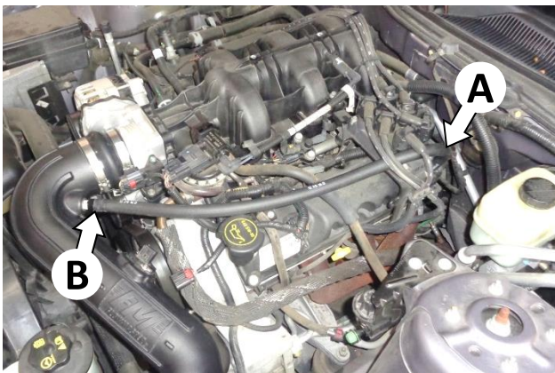
27. The hose should neither kink at the bend (A) nor chafe against the spark plug wires. Cut the hose to length and secure it to the barbed fitting (B) with the pinch clamp (24).
