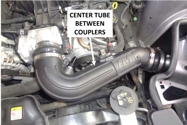
25. Center the intake tube between the couplers, and tighten the two clamps on the intake tube.
