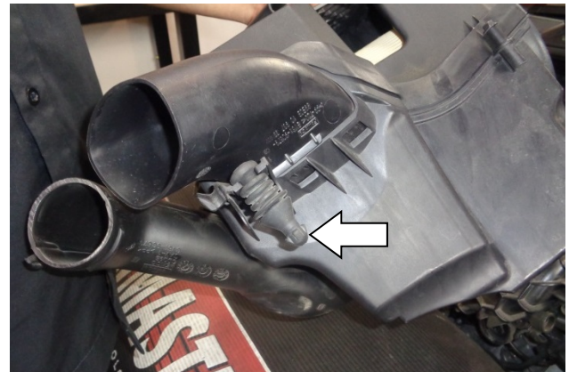
11. Remove the rubber mount pin from the airbox for use at Step 27 .
