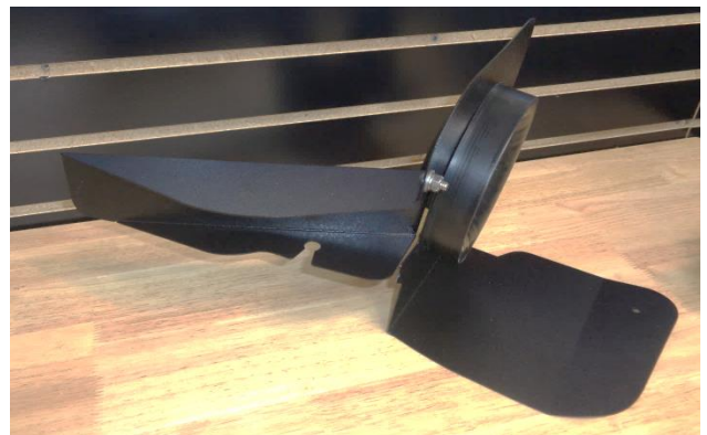
24. Assemble the inlet air duct (12) to the heat shield using a 1/4-20 screw (25) (on the duct side), and a flat washer (11), lock washer (10) and nut (9) (on the heat shield side).
