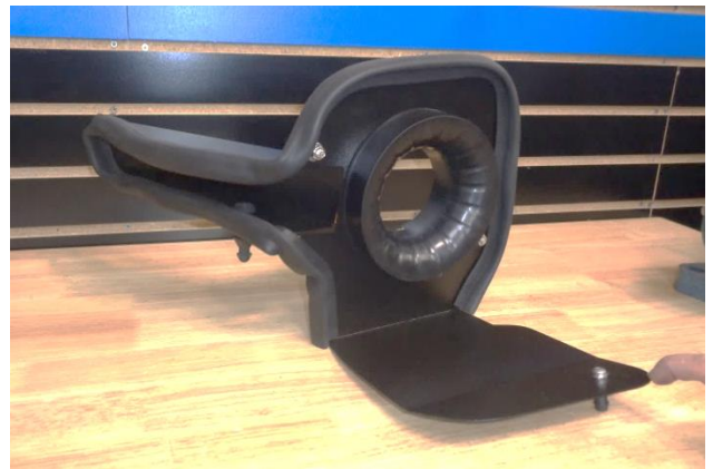
29. Attach the gasket (27) to the heat shield and inlet air duct. Starting at one end, firmly press the gasket onto the edge, gradually working around the heat shield and duct. When you reach the other end, trim the gasket to fit using metal-cutting shears.
