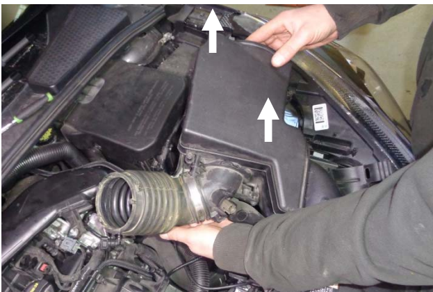
9. Pull straight up on the airbox to release its three mount pins from their grommets, then remove it from the vehicle.
