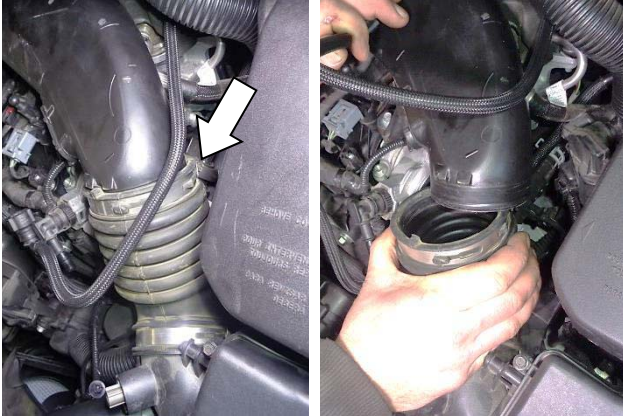
7. Loosen the screw clamp that secures the flexible duct to the rigid duct, then separate the ducts.
