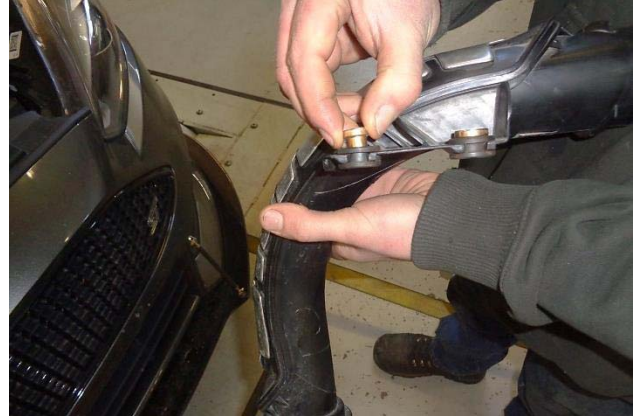
22. Remove one mount bushing from the rear inlet duct and retain it for use at Step 38 .
