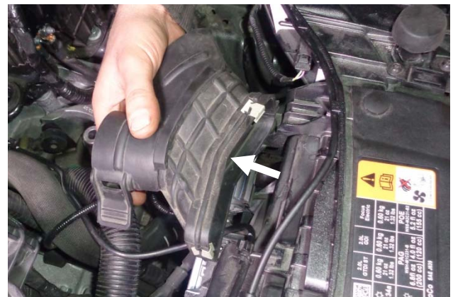
12. Pull straight back on the inlet air duct to remove it from the vehicle.
