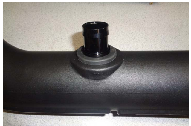
36. Push the quick-connect fitting (23) into the grommet until its flange is seated against the grommet.
