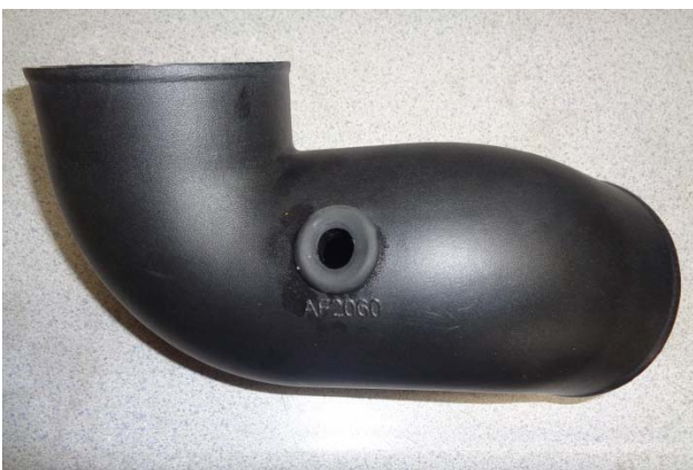
39. Insert the small rubber grommet (24) into the front intake tube (17). Moistening the grommet with soapy water will ease insertion.
