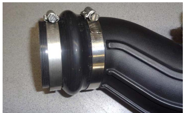
42. Install a small screw clamp (19) and a large screw clamp (15) on the large reducing coupler (18), and install the coupler on the other end of the intake tube. Do not tighten clamps at this time.
