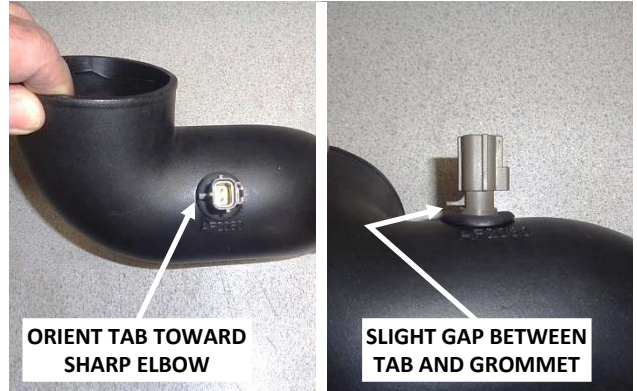
40. Carefully push the air temp sensor into the grommet, orienting the tab toward the tube's sharp elbow. Moistening the grommet I.D. with soapy water will ease insertion. NOTE: The tab does not sit flush against the grommet – there will be a slight gap.
