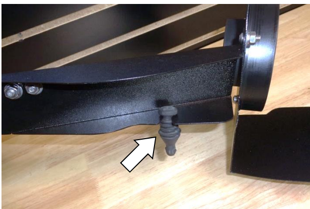
27. Push the rubber mount pin removed from the airbox at Step 11 into the notch in the inlet air duct as shown.
