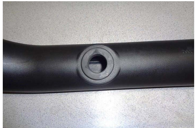
35. Insert the large rubber grommet (22) into the rear intake tube (20). Moistening the grommet with soapy water will ease insertion.
