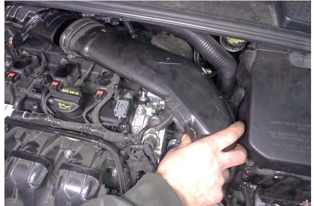
16. Separate the front duct from the rear duct and remove it from the vehicle.
