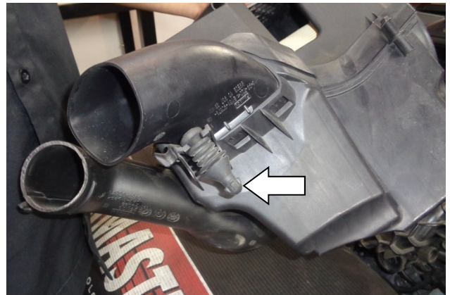
17. Remove the rubber mount pin from the airbox for use at Step 23.
