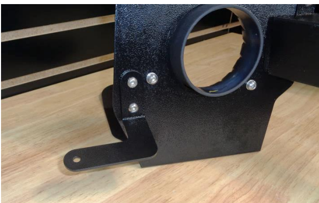
21. Attach bracket (16) to the heat shield using 1/4-20 screws (9) (on the bracket side), and flat washers (8), lock washers (7) and nuts (6) (on the heat shield side).
