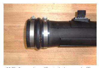
20. Slip 2 screw clamps (8) onto the large coupler (9). Push the coupler onto the filter-end of intake tube. Snug the tube clamp (do not tighten at this time), and leave the other clamp loose.
