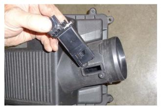
13. Remove the MAF sensor from the airbox, then remove the factory gasket from the sensor.
