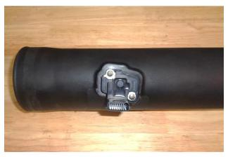
18. Install the MAF sensor gasket (13) onto the sensor, ensuring correct orientation. Then install the sensor in the intake tube, using the M4 screws (14).
