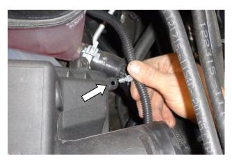
Release the clamp holding the MAF sensor wire from the corner of the airbox.
