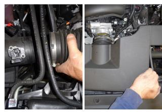
9. Separate the intake duct from the airbox, separate the intake plenum from the throttle body, and carefully remove the assembled duct and plenum from the vehicle.
