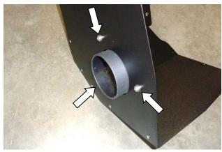
14. Assemble the air filter adapter (3) to the heat shield (4) using the M6 screws (7), lock washers (6) and flat washers (5).
