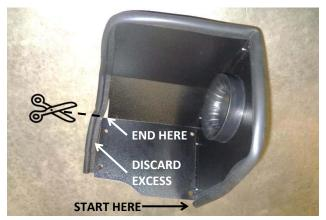
15. Attach the gasket (12) to the heat shield. Starting at the bottom of the front edge, firmly press the seal onto the edge, gradually working your way around. At the bottom of the opposite edge, trim the seal using metal-cutting shears.
