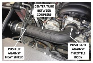
21. Install the intake tube in the vehicle. Push the rear coupler back against the throttle body and tighten the throttle body clamp. Push the left coupler up flush against the heat shield and tighten the heat shield clamp. Then center the tube between the couplers, and tighten both tube clamps.
