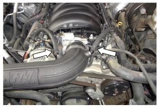
25. Push the other ends of the hoses onto the barbed elbows and secure with pinch clamps (16).
