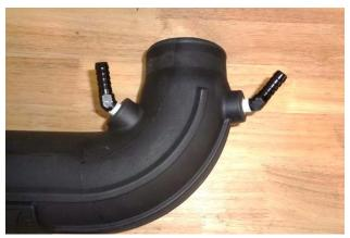
17. Apply 2 wraps of nylon thread tape to the threads of 2 barbed elbows (15), and install the elbows into the intake tube (10), pointing them toward the tube opening.
