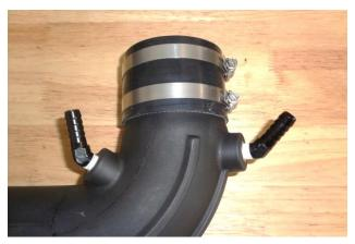
19. Slip 2 screw clamps (8) onto the small coupler (11). Push the coupler onto the throttle body-end of the intake tube. Snug the tube clamp (do not tighten at this time), and leave the other clamp loose.
