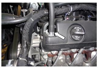
24. Install a hose on the PCV port on each valve cover (2 places). Push each hose fully onto the port, until it touches the raised lip.
