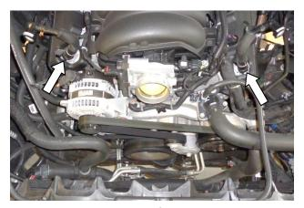
Remove both PCV hoses from the valve covers by depressing their release latches and pulling straight off.
