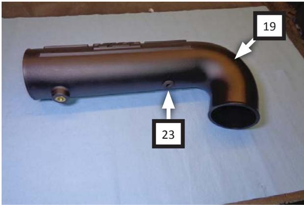
19. Insert grommet (23) into intake tube (19).
