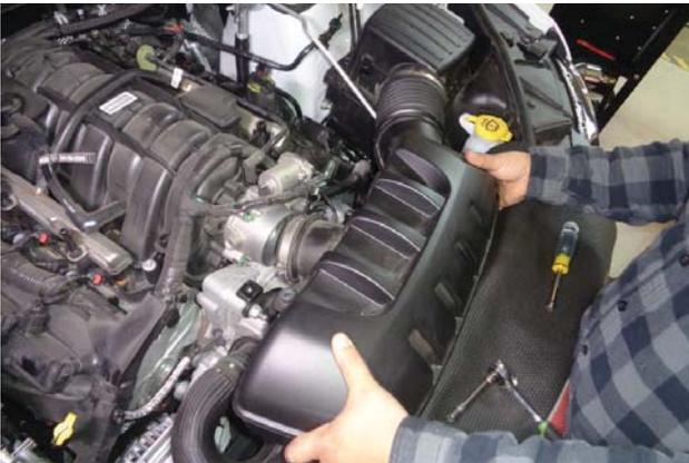
8. Remove resonator from engine compartment.
