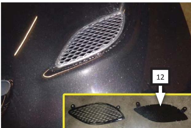
33. This step applies only to Durango RT: Re-install vent and intake block-off plate (12) in place on hood and secure using screws (removed step 32).
