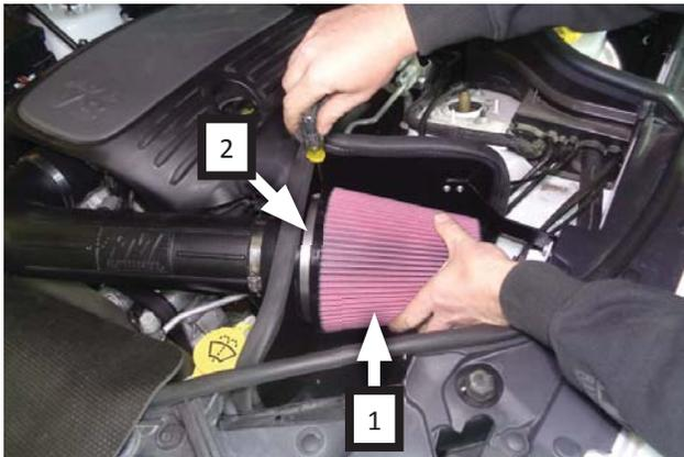
31. Place screw clamp (2) on air filter (1) then install filter onto adapter and tighten clamp.
