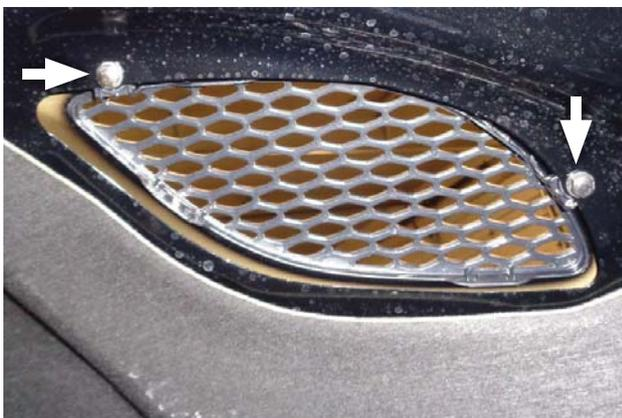
32. This step applies only to Durango RT: Remove screws and vent from underside of hood. Retain for re-use in step 33.
