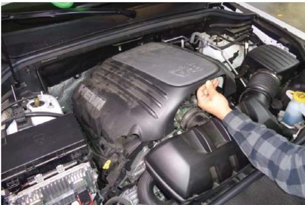
3. Lift and remove engine cover. Retain for later re-use.
