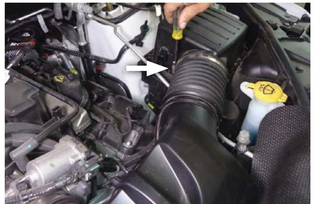
6. Loosen screw clamp then disconnect intake tube from airbox.
