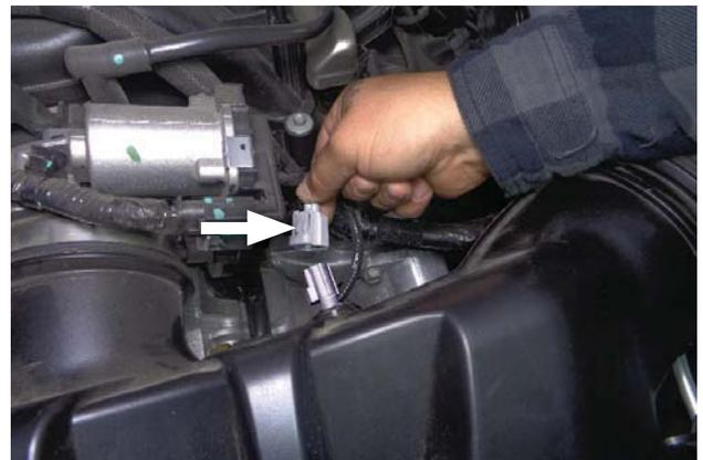
5. Unplug connector from IAT sensor on intake tube.
