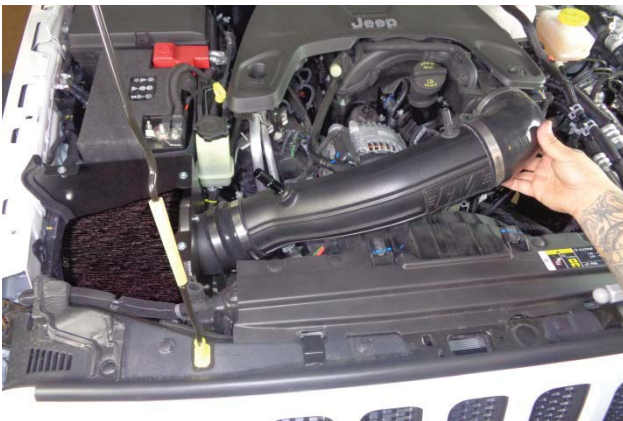
26. Install the assembled intake tube in the vehicle.
