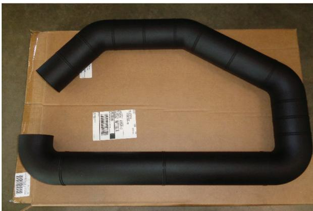
2. We have provided a **molded intake tube (1)** with multiple lengths in its configuration. This should provide enough tubing to fit most applications, you will just have to plan its route.
