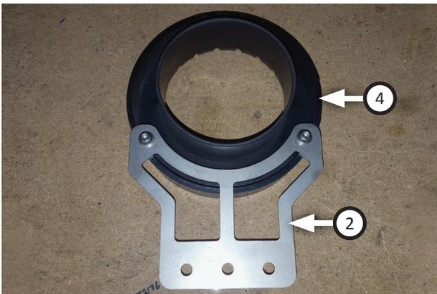
2. Install **bracket 1 (2)** onto **air filter adapter (4)** using (x2 ea.) **screws (15)**, **flat washers (17)** and **split lock washers (16)**.
