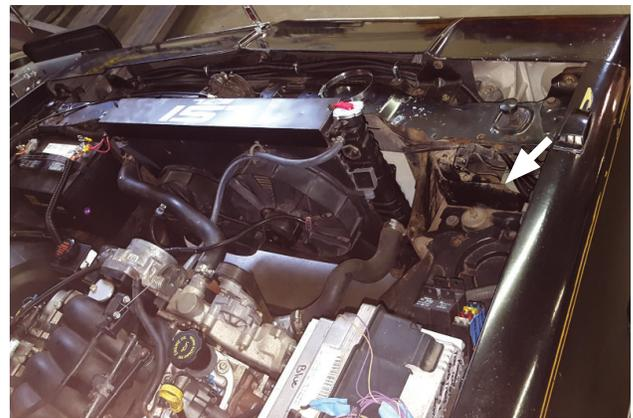
4. Decide where you would like your air filter to go. In this example, we have decided to position filter in corner behind passenger headlight where it will have an optimal amount of airflow.
