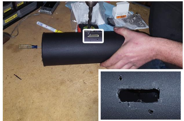
7. Disassemble parts from tube then drill marked slot for MAF Sensor. You can oversize your drill up to an  $\frac{1}{8}$ " so your MAF Sensor slides in and out easily. Deburr and smooth drilled edges.
