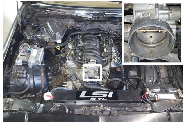
3. Identify throttle body in your vehicle, this will be the starting point for your universal air intake kit. Verify sizing then select appropriate coupler for it (very likely 3 $\frac{3}{4}$ -4").
