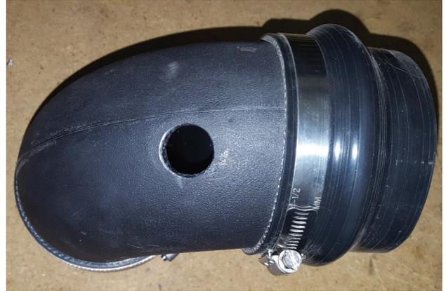
1. Remove IAT sensor from your vehicle, then use sensor to mark and drill an appropriate sized hole in your new intake system.
