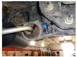
5) To simplify the installation of the new Flowmaster muffler, it may be necessary to unbolt the rear tailpipe hangers from the frame; this will give you full range of motion to get the tailpipes into the muffler outlets.
