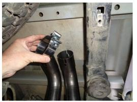
7) Place the provided 3" clamps onto the muffler outlets.
