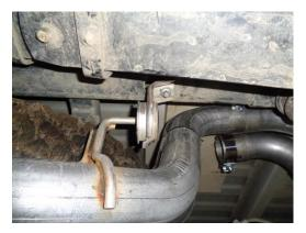
3) It may be necessary to unbolt the forward hanger on each tailpipe from the frame to allow the tailpipes to slide out of the muffler outlets.
