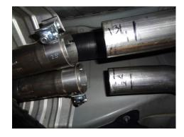
Place the left inlet pipe **#86424M** into position behind the left catalytic converter and re-install the nuts removed in the previous step. Tighten enough to hold but still allow for adjustment. Be sure to replace the gasket. Repeat the step on the right side of the vehicle with inlet pipe **#86423M**. Measure and make a mark at 1 3/4" from the back of each of the front pipes, this is the mark that the X-pipe will be slid on to.
