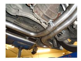
8) Place a provided clamp onto the inlets of muffler **7525554-480**. Place the muffler up into position and slide onto the intermediate pipes, make sure they are fully seated and support the muffler with a stand. Tighten the clamps enough to hold but still allow for adjustment. Place a provided clamp onto each muffler outlet.
