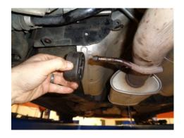
3) Remove the two nuts at the flanged connection in the center of the vehicle. Then using a ½" wrench, remove the factory mid pipe/resonator assembly hanger from the frame of the vehicle. This hanger will be replaced with hanger **385HA**. The factory rubber isolator will be re-used with the new **385HA** hanger. Lower the mid pipe/resonator from the vehicle and set aside.
