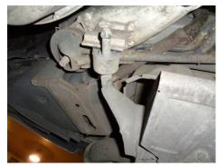
2) Support the rear muffler with a stand; use a 14MM wrench to remove the two nuts at the flanged connection in front of the muffler. Disengage the two rear hangers and the hanger at the front right corner of the muffler from the rubber mounts on the vehicle. Lower from the vehicle and set aside.
