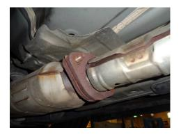
4) Using a 14MM wrench, remove the nuts at the two flanged connections behind the catalytic converters. Slide the Y-pipe rearward to disengage the front two flanges, then lower from the vehicle and set aside. Save the front two gaskets for reuse.
