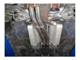
7) Using the factory nut, secure hanger #385HA to the mount on the vehicle that the factory mount was removed in step 3 above. Install the factory rubber mount. Place the intermediate pipe assembly #86455M into position and slide into the back of the X-pipe, connect the hanger on the pipe to the rubber mount on the vehicle. The hanger should be level and the rubber isolator should be vertical. Tighten the clamps enough to hold but still allow for adjustment.
