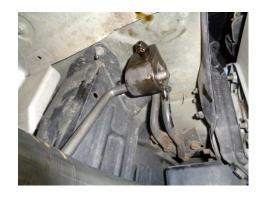
9) Place the left exit pipe **#86460M** up into position and connect the hanger on the pipe to the rubber mount on the vehicle, then slide into the muffler outlet. Adjust the exit pipe and tip to the desired position and tighten the clamp enough to hold, but still allow for adjustment. Repeat this step on the right side of the vehicle with exit pipe **#86459M**.
