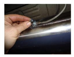
10) Using the 3/8" nut and washers included in the hardware pack attach the grounding strap above the front of the muffler to the bolt on the the new muffler. Tighten securely.
