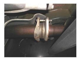
3) Support the muffler with a stand and remove the two bolts at the front flange connection. Now, with the help of an assistant, slide the exhaust system to the rear to disengage the hangers on the exhaust from the rubber mounts on the vehicle. Once free, the assembly can be removed by working it forward over the rear axle (If you are working on the ground it may be easier to cut the tailpipe off at the rear of the muffler to simplify removal).
