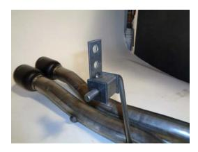
6) Slide rubber mount **#HA572** onto the end of the wire hanger of exit pipe **86467M** as shown.
