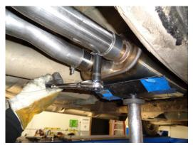
7) Place a supplied 2-1/2" clamp onto each muffler outlet. Place the exit pipe assembly **#86467M** up into position and slide into both muffler outlets approximately 2". Use a stand to support the outer end of the assembly. Tighten the clamps just enough to hold in position.
