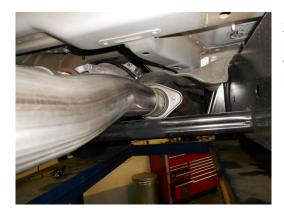
2) Place the inlet pipe onto the back of the existing OEM head pipe and fasten using the 3/8" x 2.00" bolts, nuts and washers provided in the hardware kit. Tighten just enough to hold in place, but still allow for adjustment.
