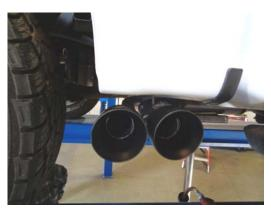
9) Adjust the position of all pipes and muffler to provide a satisfactory fit. A minimum 3/4" clearance around all parts of the system must be maintained; while also keeping suspension travel and vibration in mind.
