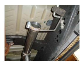
3) Slide the inlet hanger **#490HA** over the back of the inlet pipe and insert the hanger into the factory rubber mount. Do not tighten this clamp yet. **Note:** See step 4 if the frame hanger does not line up with clamp hanger 490HA.
