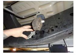
4) On some vehicles the front frame mount may be in the incorrect location to properly connect to the 490HA frame hanger. In this case, remove the two screws attaching the mount to the frame, move the two plate nuts to the forward set of holes and remount the hanger to the frame.
