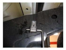
8) Adjust the exit pipe so that the tips are the desired distance from the body, then rotate the **HA572** hanger so that it lays flat against the inside of the vehicle frame and use a center punch to mark the center of the two holes on the frame. Rotate the hanger out of the way and drill each mark using a ½" drill bit. Use the two 5/16" thread cutting bolts to secure the hanger to the frame. Tighten securely.
