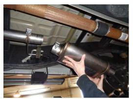
5) If required, place the extension pipe **#26277M** onto the back of the inlet pipe. Then place a supplied 3" clamp onto the muffler inlet and slide the muffler onto the inlet pipe approximately 1.75" and support with a stand. Level the muffler and tighten the clamp at the inlet enough to hold, but still allow for adjustment.
