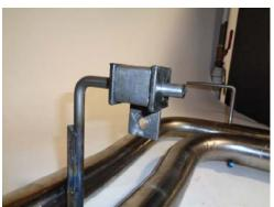
4) Place the supplied **HA602** rubber hanger onto the wire hanger closest to the tips of exit pipe assembly **#86463M**.
