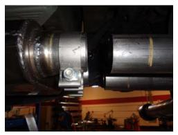
5) Place a supplied 2 ½" clamp over each muffler outlet; then place exit pipe assembly **#86463M** into the back of the muffler approximately 2". Connect the wire hanger closest to the muffler to the rubber mount on the vehicle. Tighten the clamps at the muffler outlet enough to hold but still allow for adjustment.
