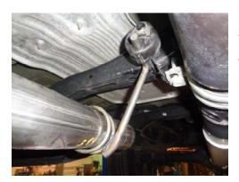
2) Place the supplied left inlet pipe clamp hanger **#384HA** and the right inlet pipe clamp hanger **#353HA** onto the inlet pipes and into the factory rubber mounts on the vehicle. Tighten clamps enough to hold in place but still allow for adjustment.
