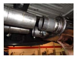
3) Place a supplied 2 ½" clamp over each muffler inlet; then slip the muffler onto the back of the inlet pipes approximately 2". Use a stand to support the muffler. Tighten clamps enough to hold in place but still allow for adjustment.
