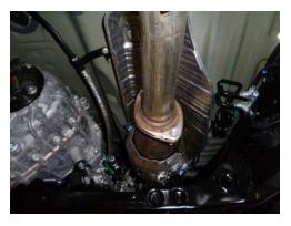
3) Support the muffler with a stand, then using a 14mm socket; unbolt the 4 bolts at the two front flanged connections. Separate the wire hangers in front and rear of the muffler from the rubber mounts on the vehicle. Remove the muffler inlet pipe assembly and set aside. Save the 4 factory bolts, they will be reused in Installation step 1.
