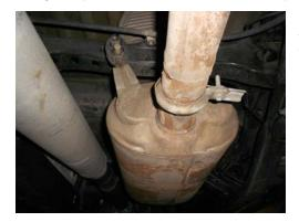
2) Using a 12mm socket, unbolt the tailpipe connection where it exits the muffler. Separate the wire hanger on the tailpipe from the rubber mount on the vehicle. Remove the tailpipe and set aside.
