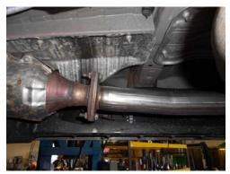
1) Place the right side inlet pipe **#86461M** and left side **#86462M** into position and fasten the flanged connections together using the bolts removed in step 3 above.
