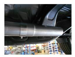
2) If installing the system on a Crew Cab truck with a 6.5' bed, place extension pipe **#TB700M** onto the back of the **#26687M** inlet pipe, place a provided clamp onto the slip-fit and tighten enough to hold in position. This extension pipe will not be used on Double Cab or Crew Cab-5.5' bed models.
