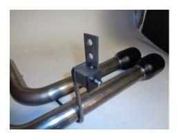
4) Slide rubber mount **#HA572** onto the end of the wire hanger of exit pipe **86465M** as shown.
