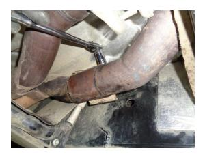
5) Support the resonator with a stand and loosen the clamp on the right inlet pipe and the two flange bolts on the left inlet pipe using a 15mm socket wrench. Then slide the resonator toward the rear of the vehicle to disconnect the inlet pipes. Lower from the vehicle and set aside.
