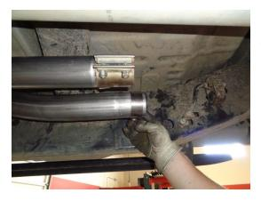
2) Place the factory band clamp from the rear of the resonator onto the left X-Pipe outlet as shown. Place the supplied 2 <sup>3</sup>/<sub>4</sub>" clamp onto the right outlet as shown.
