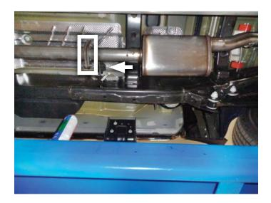
9. Secure flanges using bolt and flat washer on one side; flat washer, lock washer and nut on the other.
