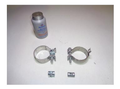
Transfer clamp from factory system onto inlet pipe (26755M) then connect it to catalytic converter. Mount wire hanger into factory isolator and tighten clamp just enough to allow for adjustment.
