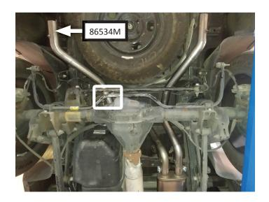
13. Place 2-½" clamps (x2) (MC250BS) onto slip fit of exit pipes (x2) (86535M). Connect exit pipes onto left rear and right tailpipes. Tighten clamps just enough to allow for adjustment.
