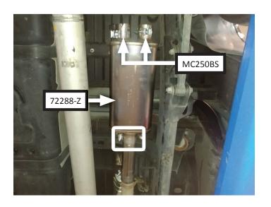
10. Route **right tailpipe (86533M)** over axle and hang rear wire hanger into factory mount. Then connect inlet to muffler outlet and hang wire hangers in factory isolators. Clip in ground wire (removed step 5). Tighten clamp just enough to allow for adjustment.
