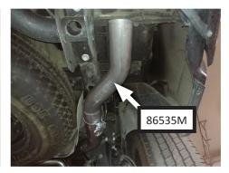
14. Place **tip (ST507B)** onto passenger side exit pipe. Secure it by fastening inlet bolt.
