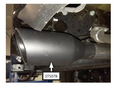
15. Place **tip (ST507B)** onto driver side exit pipe. Secure it by fastening inlet bolt.
