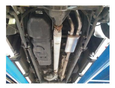
17. We recommend applying a one inch tack weld to all slipfit connections for a more secure installation. You may also apply high temperature paint over welded areas to prevent rust and premature corrosion.
