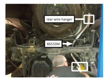
11. Remove isolator from factory mount (in step 4) and install it on left front tailpipe (86536M). Insert tailpipe wire hanger into factory mount then connect inlet to muffler. Tighten clamp just enough to allow for adjustment.
