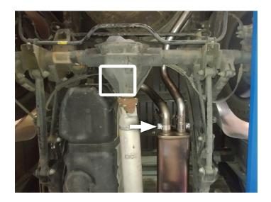
12. Place 2-½" clamp (MC250BS) onto left rear tailpipe (86534M) intlet. Insert left rear tailpipe wire hanger into factory isolater then connect inlet to left front tailpipe. Tighten clamp just enough to allow for adjustment.
