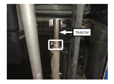
Place 3" clamp (MC300BS) onto muffler (72288-Z) inlet then connect muffler to adapter pipe. Place 2-½" clamps (x2) (MC250BS) onto muffler outlets. Tighten front clamp just enough to allow for adjustment.
