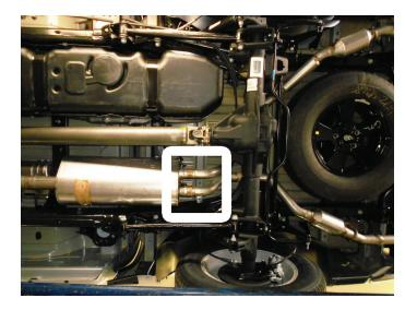
4. Dismount tailpipes from factory isolators (x3) and remove them from vehicle.
