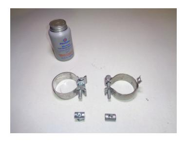
Place 3" band clamp (MC300BS) onto adapter pipe (TB467M) inlet. Connect adaper to factory pipe; line up notch in adapter with tab on factory pipe then slide them together. Tighten clamp just enough to allow for adjustment.
