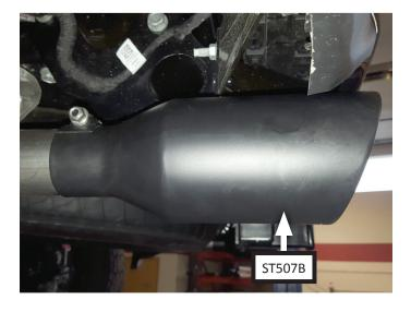
16. Adjust exhaust components to provide a satisfactory fit. Maintain a minimum of 1/2" clearance around all components of the exhaust system, keeping in mind suspension, travel and vibration. After making any required adjustments, securely tighten clamps.
