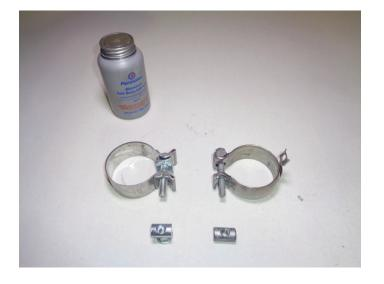
Place (x2) ball clamps (removed step 4) onto left (1) and right (2) mufflers then install them onto vehicle, inserting wires into isolators. Tighten clamps just enough for later adjustment.
