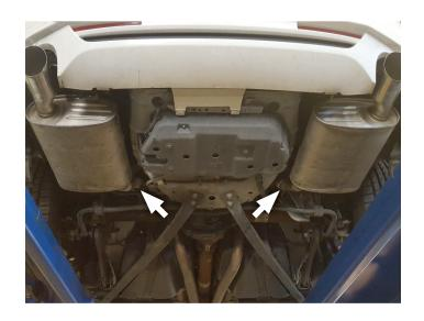
4. Slide wire hangers out of isolators then remove both mufflers from vehicle. Remove and retain ball clamps for later use.
