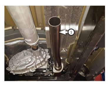
10. Fasten inlet using (x2 ea.) bolts (11), flat washers (13), lock washers (14) and nuts (12).
