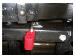
14. Fasten backing plate (HA566), flat washer (HW303), lock washer (HW309) then nut (HW103) onto screw on back side of vehicle frame. Center assembly in oblong hole then tighten completely.
