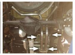
12. Place clamp (MC250BS) onto right rear tailpipe (86545M) then connect it to right front tailpipe. Hang wire hanger into isolator then tighten clamp enough to allow for adjustment.
