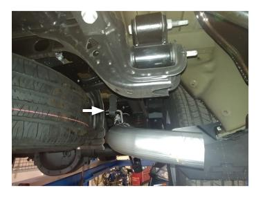
13. Insert screw (HW220), left frame hanger (226HA), backing plate (HA566) and rubber hanger (HA168) into oblong hole on vehicle frame behind rear driver tire as shown.
