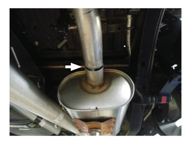
4. Dismount tailpipe from isolators (x3) then remove from vehicle.
