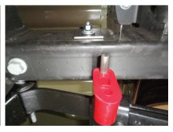
Place clamp (MC250BS) onto left rear tailpipe (86544M)
