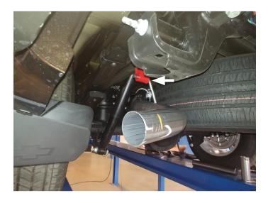
16. Place **tips (ST507B)** onto rear tailpipes. Tighten inlets to secure connection.
