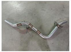
5. Dismount inlet exhaust pipe from mount. Loosen clamp from catalytic converter connection then remove remaining exhaust assembly from vehicle. Remove and retain clamp for later use.
