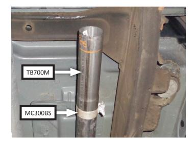
10. Place 3" clamp (MC300BS) onto muffler (72288-Z) inlet. Place 2-½" clamps (x2) (MC250BS) onto muffler outlets. Connect muffler to inlet or extension pipe then tighten front clamp just enough to allow for adjustment.
