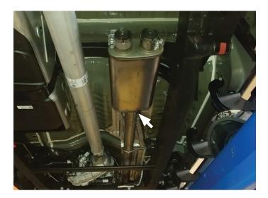
11. Route right front tailpipe (86543M) and left front tailpipe (86542M) over axle and connect them to muffler outlets. Mount wire hangers into isolators then tighten clamps (x2) enough to allow for adjustment.
