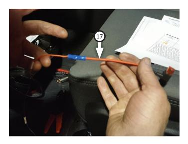
18. Pull factory fuse from F66 (Run - Accessory Feed) in fuse box. Plug it and **fuse (16)** into fused circuit tap, route wire over to fuse box then plug it back into F66 as shown. Secure any wire slack up and out of the way.
