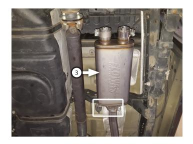
10. Route **right tailpipe (6)** and **left front tailpipe (4)** over axle and connect them to muffler outlets. Mount wire hangers into isolators then tighten clamps (x2) enough to allow for adjustment.
