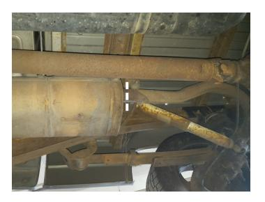
4. Remove O<sup>2</sup> sensor from front pipe by first unplugging wire at clip connection, then unscrewing sensor from fitting on pipe.
