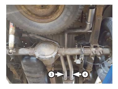
12. Place **clamp (11)** onto **left rear tailpipe (5)** then connect it to left front tailpipe. Insert wire hanger into rubber hanger then tighten clamp just enough to allow for later adjustment.
