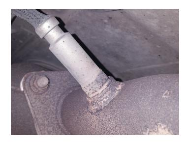
5. Support muffler and disassemble remaining wire hanger from isolator. Then remove nuts (x3) at muffler to catalytic flange connection and remove exhaust system. Retain nuts for later use.
