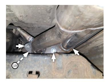
9. Place clamp (10) onto muffler (2) inlet then connect it to cat pipe assembly. Tighten clamp just enough to allow for adjustment then place clamps (x2) (11) onto muffler outlets.
