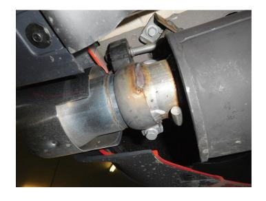
6. Remove (x3) nuts securing actuator to mounts on tailpipes. Remove actuator and spring from mount on each tailpipe.
