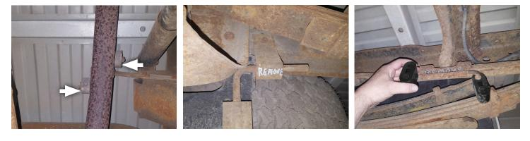
5. Remove clamp on muffler inlet, then remove muffler and set aside.
