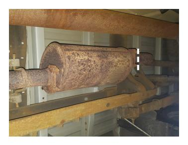
4. Separate wire hangers from isolators behind muffler. Remove bolt and hanger connecting stock tailpipe to vehicle frame (as shown, depending on your application). Remove tailpipe section from vehicle.
