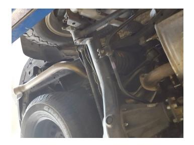
4. Support muffler and disassemble wire hangers from isolators. Remove and retain (x2 ea.) fasteners from flange connecting muffler to inlet then remove muffler section from vehicle.
