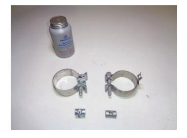
7. Place clamp (4) onto right muffler (1) then insert its wire hanger into front rubber hanger and connect it to front pipe. Re-install rear rubber mount (removed step 4). Repeat step with left muffler (2) and clamp (4).
