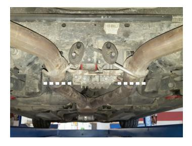
4. Support muffler then remove it from front rubber hanger mounts. Slide muffler forward to disengage and remove it. Remove and retain rear rubber mounts. Repeat procedure for remaining muffler.
