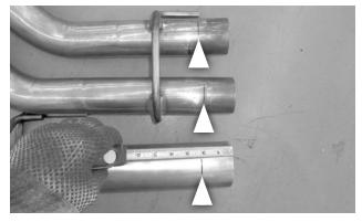
**11.** Each pipe must be inserted approximately 2" into the muffler. Mark each pipe 2" from its end to ensure proper insertion during assembly.
