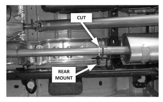
5. Cut the inlet pipe off just forward of its rear hanger rod (so that the rod remains with the muffler). Remove the muffler by pulling the hanger rods out of their isolators.
