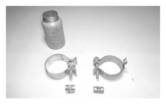
**9. Remove the nuts from the four clamps,** apply anti-seize compound to the bolt threads, and re-install the nuts.
