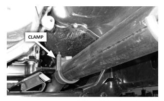
**NOTE:** The clamp may need to be cut, and the inlet pipe will likely need to be heated, to remove the pipe.
