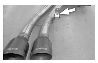
**14. Install universal bracket (6)** onto the rear hanger rod on **tailpipe assembly (3),** with the flat facing away from the tailpipe tips.
