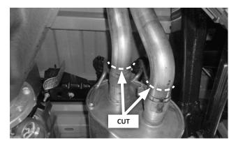
**2. Cut the tailpipe(s) off** just behind the muffler clamp(s).
