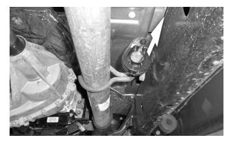
**6. Pull the inlet pipe's front isolator mount off** of the frame and pipe hanger rods.
