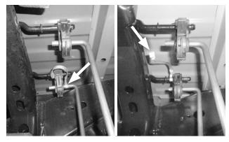
If you find a bonding strap between the frame and muffler hangers during disassembly, unclip the mufflerend of the strap.
