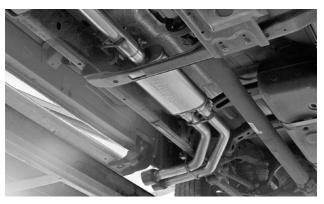
17. Adjust all components to give 1/2" to 3/4" clearance (a finger's width) around them, and allowing for suspension travel and vibration. When you are satisfied with the system's clearance and fit, tighten the four clamps. If you disconnected any frame-to-exhaust bonding wires at Step 4, reconnect them now (relocate if required).
