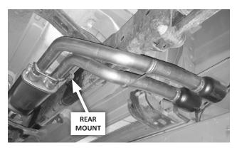
**15. Slip two 2-1/2" clamps (5) over the muffler outlets.** Insert the tailpipe assembly's hanger rod in the rear isolator mount, insert both pipes 2" into the muffler, and snug the clamps.
