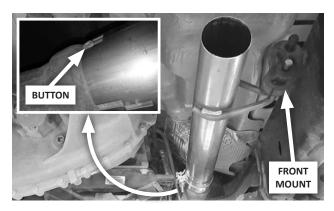
12. Slip one 3" clamp (4) over the front of the inlet pipe. Align the notch at the front of the pipe with the button on the stock Y-pipe, and slide the inlet pipe fully onto the Y-pipe. Install the front isolator mount on the pipe and frame hanger rods. Slide the clamp over the end of the pipe, and snug it slightly (just enough to allow final adjustment later).
