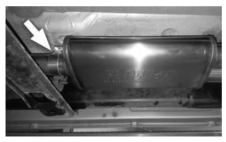
13. Slip the second 3" clamp (4) over the muffler (2) inlet. Then install the muffler on the rear end of the inlet pipe and support it with a stand. Verify 2" of insertion, and snug the clamp.
