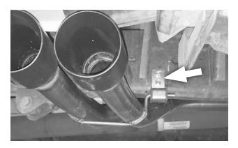
16. Adjust the tailpipe assembly so that the pipes clear the frame, and the tips are set at the desired distance from the body. Lay the bracket flat against the truck's frame, then mark its hole locations on the frame. Move the bracket aside, drill a 1/4" hole at each mark, and secure the bracket to the frame with the two thread-cutting screws (7).
