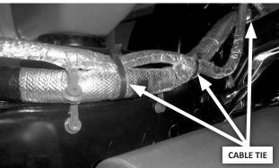
**8.** If there is a wire loom routed along the inner face of the right frame near the muffler's location, unclip the harness from the frame, then cable tie it to top of the frame (or to the wire loom already on top of the frame).
