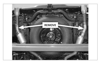
3. Release the tailpipe hanger rods from their rubber isolators, and remove the tailpipe(s) from the vehicle.
