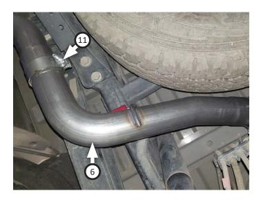
13. Place (x2 ea.) clamps (11) onto side exit pipes (7) then connect them to tailpipes and tighten clamps just enough to allow for later adjustment.
