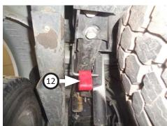
Route right (4) and left front (5) tailpipes over axle then connect them to muffler. Insert their wire hangers into isolators then tighten clamps just enough to allow for adjustment.
