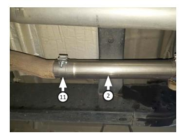
8. Place clamp (11) onto inlet pipe (1) then connect it to resonator pipe or factory pipe, lining pipe notch up to front pipe tab. Insert wire hanger in isolator and tighten clamp enough to allow for adjustment.
