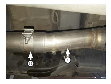
9. Place clamp (10) onto muffler (3) then connect it to inlet or resonator pipe. Tighten clamp just enough to allow for adjustment. Place (x2) clamps (8) onto muffler outlets.
