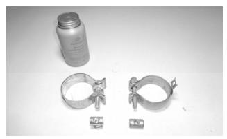
**4. Remove the nuts from all of the clamps,** apply anti-seize compound to the bolt threads, and re-install the nuts.
