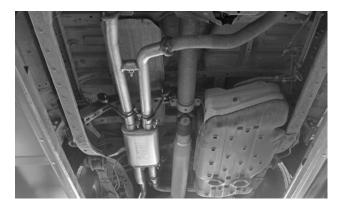
**12.** Adjust all components to obtain 1/2" to 3/4" clearance (a finger's width) around them, and to allow for suspension travel and vibration. When you are satisfied with the system's clearance and fit, tighten all seven clamps.
