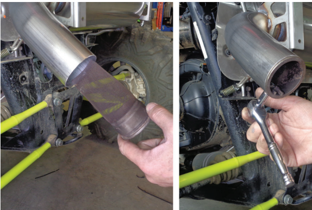
14. Install nut, bolt and spark arrestor (removed step 8) into end of muffler.
