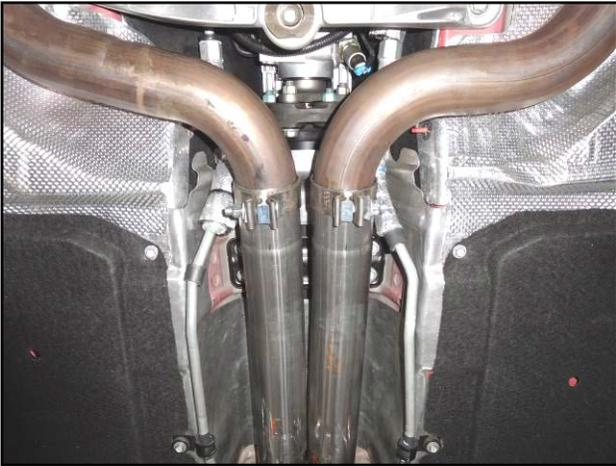
1) Place a supplied 2 3/4" clamp onto the inlets of Scavenger assembly **#26611S**, place the assembly onto the front inlet pipes and slide on approximately 3.00". Be sure the Flowmaster embossing in the center of the assembly is facing the ground. Re-install the body brace and tighten securely.
