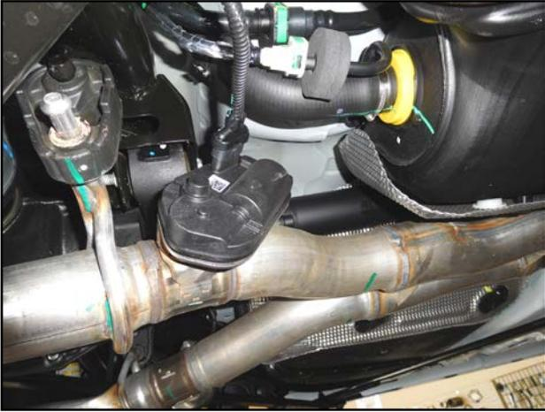
4) Just forward of the rear axle there is an exhaust valve integrated into each exhaust pipe. Using a 10mm wrench, remove the three bolts securing each of the electronic actuators to the valve. Set the bolts aside and tuck the actuator up out of the way for reinstallation on the new Flowmaster mid pipes. **Note:** On vehicles equipped with the Dual Mode Exhaust option, repeat this step with the second set of valves located on the exit pipes at the rear of the vehicle.
