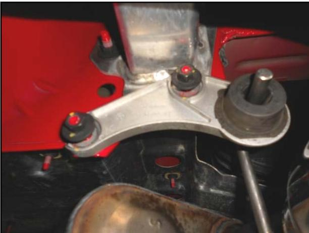
2) Support the rear of the system with a stand and using a 15mm socket or wrench, remove the two hangers at the rear of the system.
