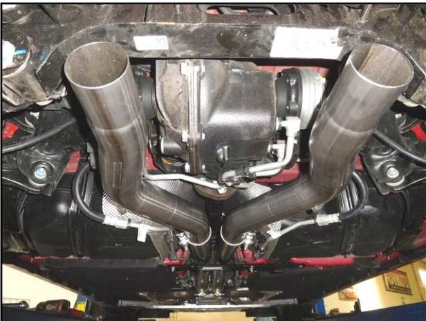
2) Place a provided 3.00" clamp onto the slip-fit of mid pipe **#26616S** and slide onto the back of the left side Scavenger outlet. Connect the hanger on the pipe to the rubber mount on the vehicle and tighten the clamp enough to hold in place. Repeat this step on the right side of the vehicle with mid pipe **#26618S**. You can now follow the installation section of the instructions provided with your new Flowmaster axle-back system.
