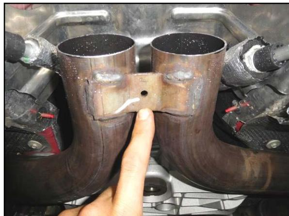
6) Carefully deburr the ends of the front pipes where cut with a file or die grinder. The next step will be to remove the brace between the two front pipes. See the two photos above.
