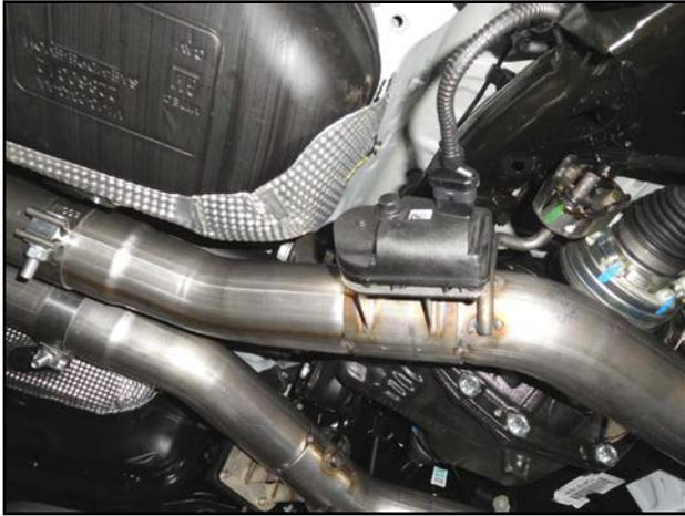
3) Locate the exhaust valve actuators removed in step 4 of the removal instructions and place onto the valves in the new Flowmaster mid pipes. Using the factory bolts and washers, securely fasten the actuators to the valves. **Note:** On vehicles equipped with the Dual Mode Exhaust option, repeat this step with the second set of valves located on the exit pipes of the new Flowmaster muffler assemblies.
