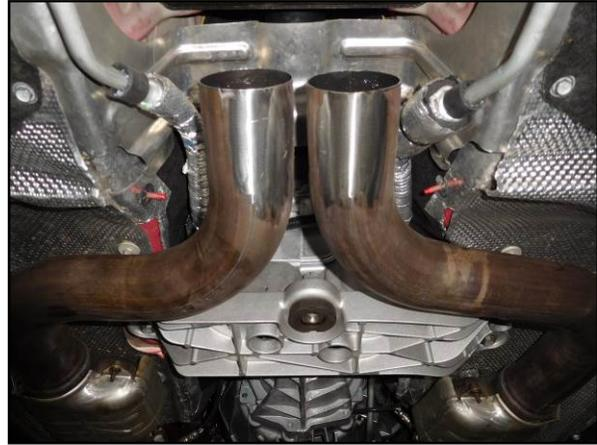
7) Using a grinder, grind down the welds on either end of the brace, the welds must be completely removed in order for the new Scavenger assembly to slide on smoothly.
