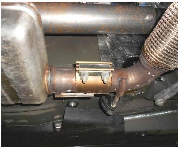
3) Using a 15mm wrench, loosen the two bolts at the clamp connection in the center of the vehicle. Use a small screwdriver to lift the clip and with the help of an assistant, carefully lower the stands at the rear of the resonator and slide the system toward the rear and off of the front pipe. Lower the resonator from the vehicle. The clamp should remain on the factory front pipe as it will be re-used with the new Flowmaster system.
