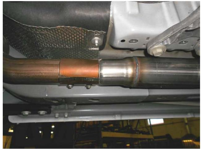
1) Be sure that the factory band clamp from the resonator inlet is in place on the front pipe behind the catalytic converters. Place the Y-pipe assembly **#86320S** up into position behind the factory front pipe and slide into the clamp until it stops. Support the rear of the Y-pipe with a stand and tighten the clamp enough to hold, but still allow for adjustment. The Y-pipe outlet with two bends will be oriented to the drivers' side of the vehicle.
