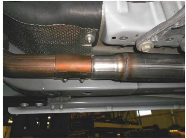
2) Be sure that the factory band clamp from the resonator inlet is in place on the front pipe behind the catalytic converters. Place the Y-pipe assembly **#86320S** up into position behind the factory front pipe and slide into the clamp until it stops. Support the rear of the Y-pipe with a stand and tighten the clamp enough to hold, but still allow for adjustment. The Y-pipe outlet with two bends will be oriented to the drivers' side of the vehicle.
