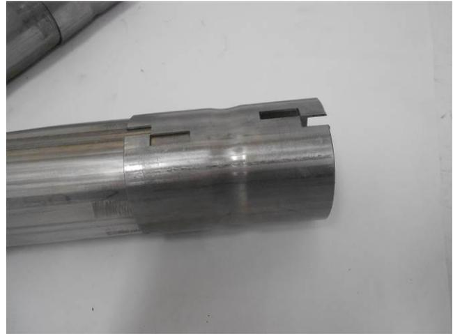
1) When using the **#86320S** Y-Pipe assembly with the factory Mustang mufflers, you must first trim 2.50" from the end of both pipes at the back of the assembly. Make a mark 2.50" from the end of both pipes and cut using a hacksaw or sawsall. Use a file or die grinder to remove any burrs from the pipe ends. After cutting, slide on the **TB810S** adapter pipes onto the end of each outlet pipe. Place a supplied clamp onto the connections and tighten enough to hold.
