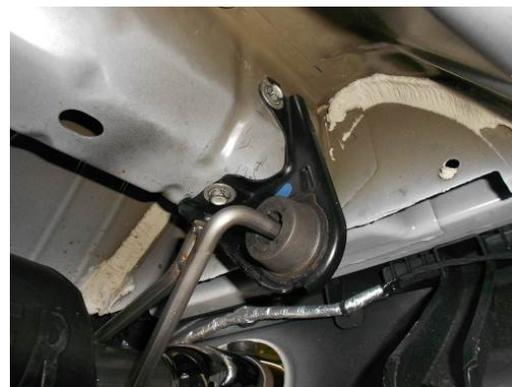
3) Using a 13mm wrench, loosen the two hangers just behind the rear differential from the cross member and the two hanger mounts at the rear of the vehicle from the frame. Slide the muffler assemblies toward the rear of the vehicle to disengage them from the factory system. Leave them hanging in place for re-assembly onto the Flowmaster Y-pipe assembly.
