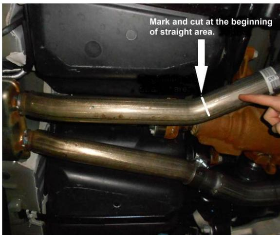
2) Begin by marking both resonator exit pipes at the beginning of the straight area as shown in the photo at left. Support the exhaust system both in front and behind the area to be cut. Check that the marks are correct, then using a sawsall, cut both pipes at the marks. **Note: Due to the closeness of the pipes to the gas tank, use caution when cutting!** Carefully deburr the end of the muffler inlet pipes where cut with a file or die grinder.
