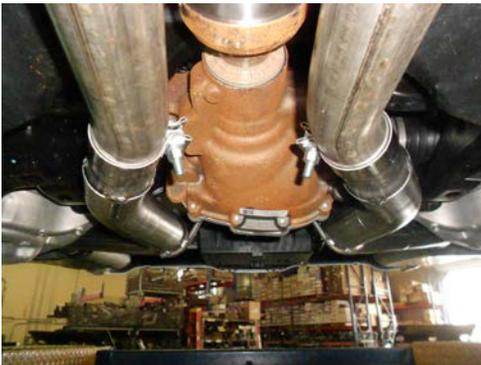
2) Place a stand under the center resonator just forward of the axle-back muffler assemblies. Loosen the clamps at the inlets of the Flowmaster or Hurst axle-back mufflers.
