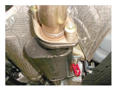
Place clamp (7) onto left muffler (4) then connect it to scavenger, inserting wire hanger into isolator. Tighten clamp just enough to allow for adjustment. Repeat this on passenger side with right muffler (5).
