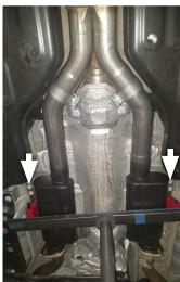
9. Secure resonator flange with (x2 ea.) **bolts (8)**, **spacers (9)**, **washers (12)**, nuts and springs (removed step 3) as shown. Repeat this step on remaining resonator flange.
