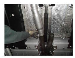
6) Place a supplied 3" clamp onto the inlet neck of both mufflers. Slide the mufflers onto the back of the Scavenger pipe assembly and support with stands. Level the mufflers and tighten the clamps enough to hold, but still allow for adjustment.
