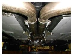
5) Begin the installation by placing a supplied 2-3/4" clamp onto each of the inlets of the Scavenger pipe #26522S. Then place the Scavenger pipe onto the back of the stock head pipes (the offset outlet pipe should be oriented to the right side). Level and center the assembly in the drive line tunnel and support with a stand. Tighten the two clamps enough to hold, but still allow for adjustment.
