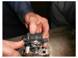
4) Be sure that the center arm of the actuator spring is between the bottom and top tabs of the mount, tighten all three bolts securely. Repeat the step on the other tailpipe assembly.
