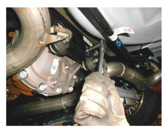
2) Support both of the mufflers at the rear of the system with a stand. Then using a 13mm wrench, unbolt the two hangers located just behind the rear differential from the cross member, leave them attached to the factory exhaust system. Again using a 13mm wrench, unbolt the hangers at the rear of the vehicle from the frame and leave attached to the system.
