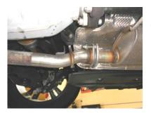
Using a 13mm socket, unbolt the left tailpipe assembly at the flanged connection at the rear of the muffler. Slide the three hanger rods out of the rubber mounts on the vehicle and remove the left tailpipe assembly.
