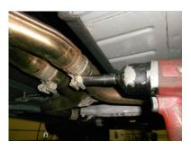
Support the rear of the system with a stand, then starting at the rear of the vehicle remove the three hangers on the right side of the system from the rubber mounts on the vehicle. Unclip the ground strap from the middle hanger on the right tailpipe and using a 15mm socket, loosen the clamps at the slip fit connections behind the catalytic converters. Then with the help of an assistant, lower the stand and slide the system back off of the head pipes. Carefully lower from the vehicle.
