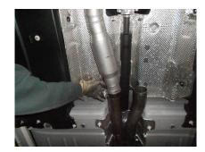
3) Place a supplied 2 ½" clamp onto the inlet of each #815425-460 muffler. Then fully slide the mufflers onto the back of the Scavenger pipe assembly and support with stands. Level the mufflers and tighten the clamps enough to hold, but still allow for adjustment.
