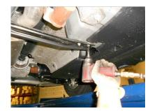
Using a 13mm socket, unbolt the two body braces in the center of the vehicle and set aside. The braces will be re-installed after completing step 2 of the installation instructions below.
