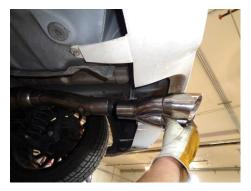
8) Place the **ST455** stainless tip onto the back of the resonator assembly and adjust to the desired position. Tighten the pinch bolt on the tip enough to hold but still allow for adjustment.
