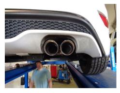
9) Adjust the position of all components to provide a satisfactory fit. This is a tight fitting system, so take your time and be patient, tightening and adjusting a little bit at a time. Be sure to maintain an adequate clearance around all parts of the system to avoid rattles or damage to heat sensitive components. Once you're happy with the fit, tighten all connections down securely. For a cleaner appearance and more secure installation, we highly recommend welding all slip-fit connections.
