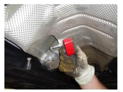
4) Place the provided **HA1640** polyurethane hangers onto each of the four factory hanger mounts on the vehicle.
