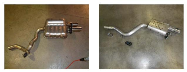
1) Place the new Flowmaster muffler units next to the factory units and swap the front and rear hanger mounts from the stock mufflers to the new mufflers. Also, place a provided 2.50" clamp onto the inlet of each assembly. Tighten the clamp just enough to hold in place.
