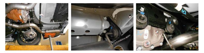
7) Place the right muffler assembly **#853063-481** up into position and slide onto the factory pipe approximately 2½". Support the assembly with a stand and remount the rear hanger mount to the frame and tighten securely. Remount the front hanger to the cross member and tighten securely. Leave the clamp on the inlet loose for now. Repeat this step with muffler assembly **#853063-482** on the left side of the vehicle.
