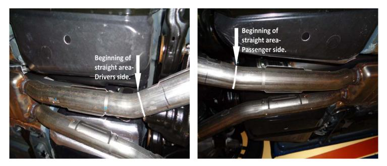
4) Behind the factory center resonator, follow the pipes back just past the second bend of each pipe, make a mark on each pipe where the bend ends and the straight area begins. See above photos. At the rear of each muffler unplug the wire to the factory exhaust actuator and tuck the connection up out of the way until ready to re-connect to the new mufflers.
