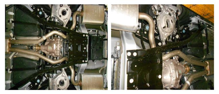
2) On convertible model vehicles, the body braces shown in the photos above will need to be removed in order to remove the factory system and install the Flowmaster system. Starting at the front of the right side (passenger) brace, loosen the front bolt and then work your way to the rear of the vehicle removing the next eight bolts, lower the brace from the vehicle. Repeat this step on the left side of the vehicle with the six bolts on that side.
