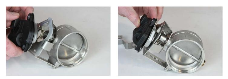
4) **Installing the actuator onto the new valves:** Line up the spring arm with the notch in the valve shaft and lower into place. The holes in the actuator assembly should line up with the holes in the mount, rotate if required.
