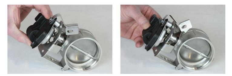
5) Place a supplied 1/4" Button head screw thru the grounding clip removed from the stock valve and then into the hole on the opposite side of the FM in the mounting plate. Place a supplied  $\frac{1}{2}$ " spacer between the mount and the actuator heatshield, then follow with a supplied lock washer and nut on the bottom side of the mount.
