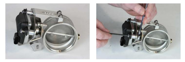
6) Use the remaining <sup>1</sup>/<sub>4</sub>" hardware to secure the actuator to the mount in the remaining two holes. Tighten securely using a 7/16" open end and 5/32" Hex wrench.
