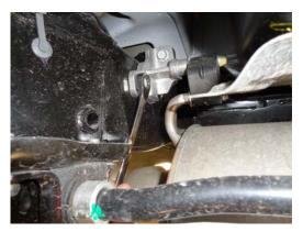
3) Locate the left and right rear mounts supporting the muffler, use a 13MM open end wrench to remove the lower bolt on each mount.
