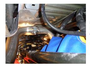
1) Place the supplied clamp onto the inlet of the new Flowmaster muffler, then place the muffler up into position and slide the inlet onto the factory over-axle pipe. Line up the notch in the inlet pipe with the tab on the over-axle pipe, slide on completely. Support the muffler with a stand.
