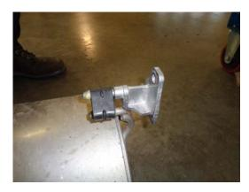
5) Place the factory muffler next to the new Flowmaster muffler and move the factory hanger mounts onto the wire hangers of the new muffler.
