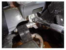
4) Then, use a 13MM socket wrench to remove the upper bolt on each mount. Once both hangers are un-fastened, carefully lower the stand and with the help of an assistant slide the muffler off of the inlet pipe and remove from the vehicle.
